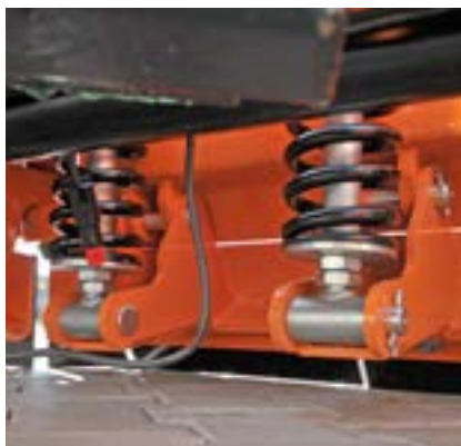
Spring shock absorption of the blade
