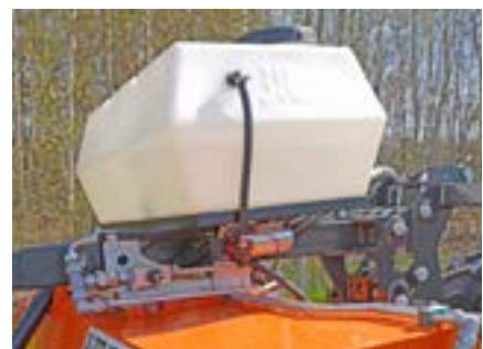
Additional water tank
