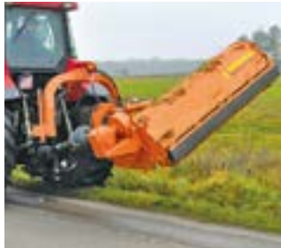
Hydraulic adjustment of the working angle
