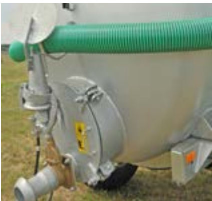
Drain connection at the lowest point of the tank
