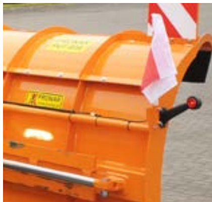
Position marking lights
