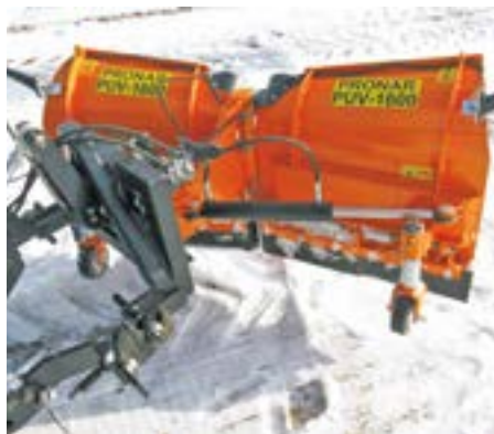
Electrohydraulic adjustment of the working angle
