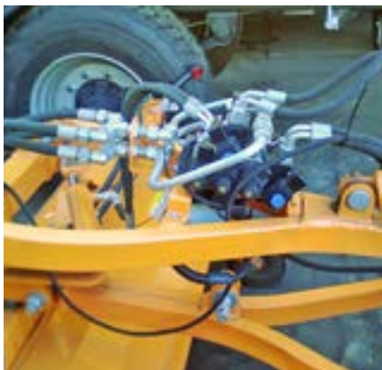
Hydraulic brush rotation \pm 30^\circ
