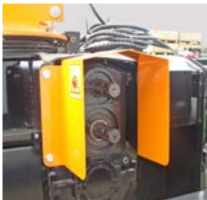
Transmission with two PTO outputs (rear-540 / front-1000 rpm)
