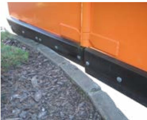
Spring shock absorption of the blade
