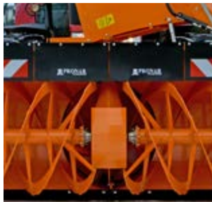
Snail-cutter for cutting frozen snow and ice. Working height of 1.245m
