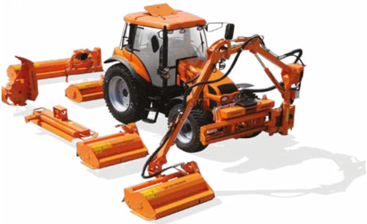
WWP600 multifunction arm with GP200 saw for branch cutting
