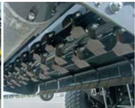
Cutting unit - cutting shaft with replaceable knives
