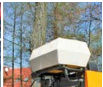
Additional water tank (200 l)
