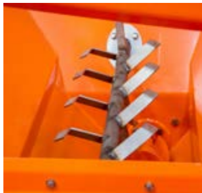
Additional mixer facilitates aggregate breaking
