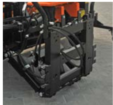
Mounting - DIN type A municipal plate
