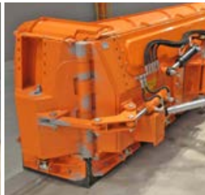
Hydraulic adjustment of the wing position in the range of -60° to +90°
