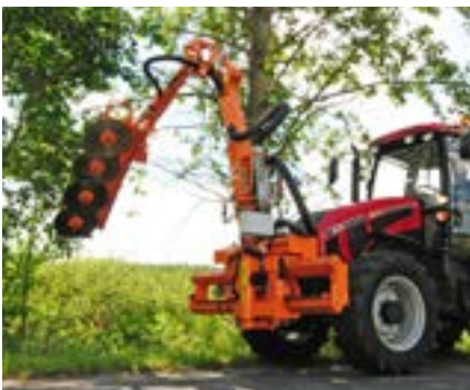
WWP600 multifunction arm with GP200 saw for branch cutting
