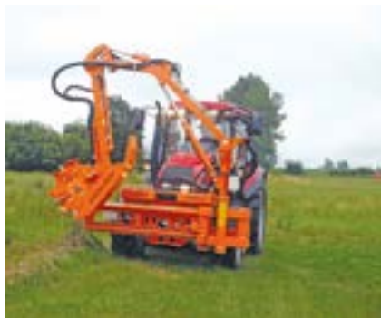
WWP600 with GO800 ditch digger. Long reach fits perfectly for desludging
