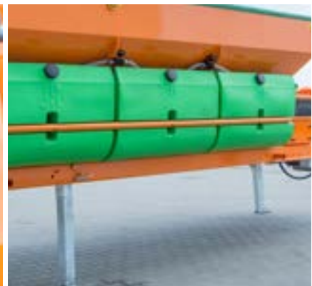
RORO (Roll-on / Roll-off) system for easier loading of PT70 spreader on the carrier platform
