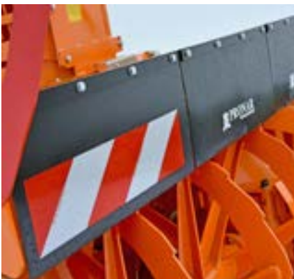
Rubber covers protect against dusting
