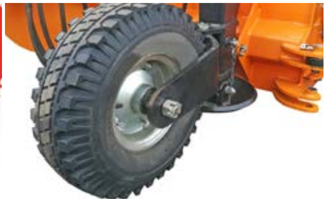
Slides and support wheels to maintain the distance between the surface and the blades (to limit the thickness of the swept layer)
