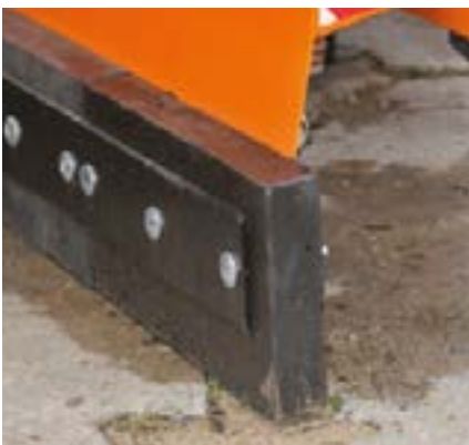
Rubber blades with shock absorption
