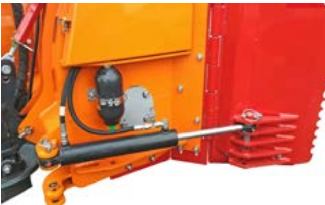
Hydraulic control of the widening
