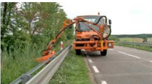
Mowing of a hard-to-reach roadside using a WWP500U multifunction arm and GK 110 head
