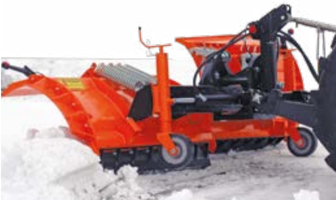
Segmented mouldboard with spring safeguard
