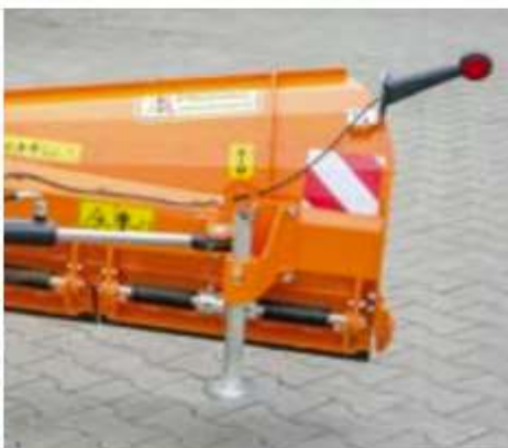
Split working blades
